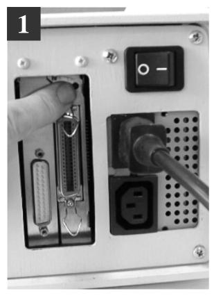
At the rear of the printer, locate the TEST Push-button. This is located in the rear panel, just above the Centronics parallel interface connector.
